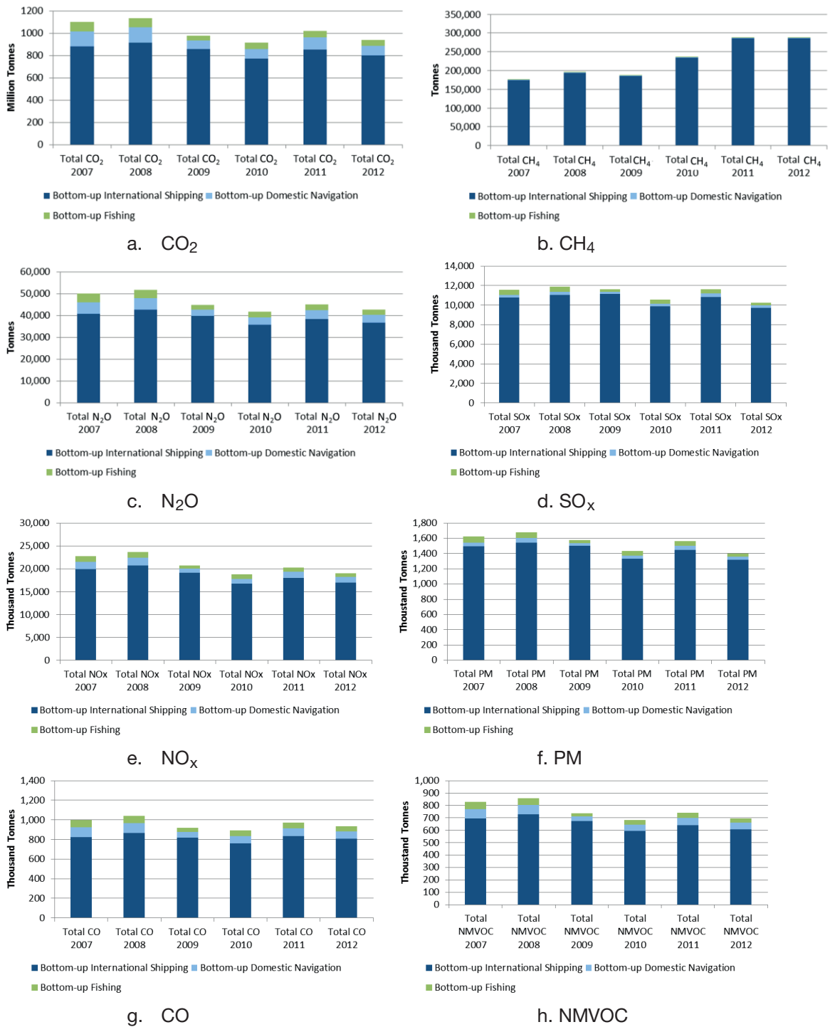
Figure 10: Time series of bottom-up results for GHGs and other substances (international shipping, domestic navigation and fishing)
